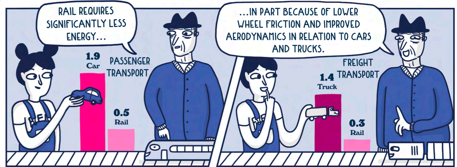
Comparison of energy consumption between road and rail (in megajoules* per passenger or ton kilometer*, 2017)
