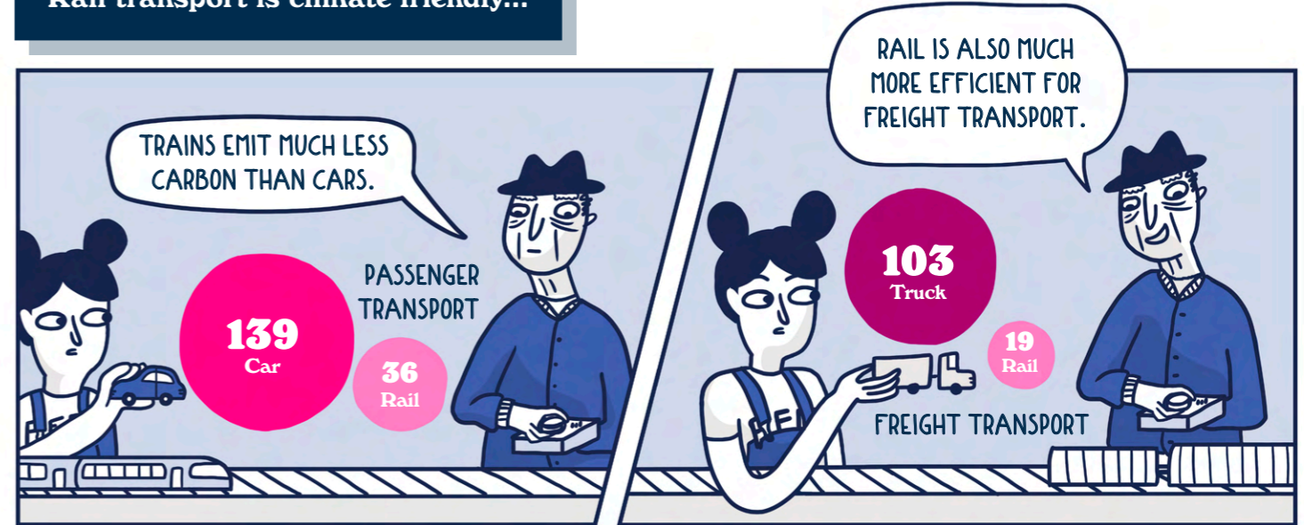
Comparison of greenhouse gas emissions between road and rail (in gram CO 2 equivalents per passenger or ton kilometer, 2017)
